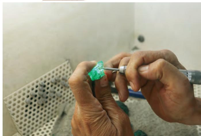
Recovery station: cleaning emerald crystal using pneumatic chisel.
