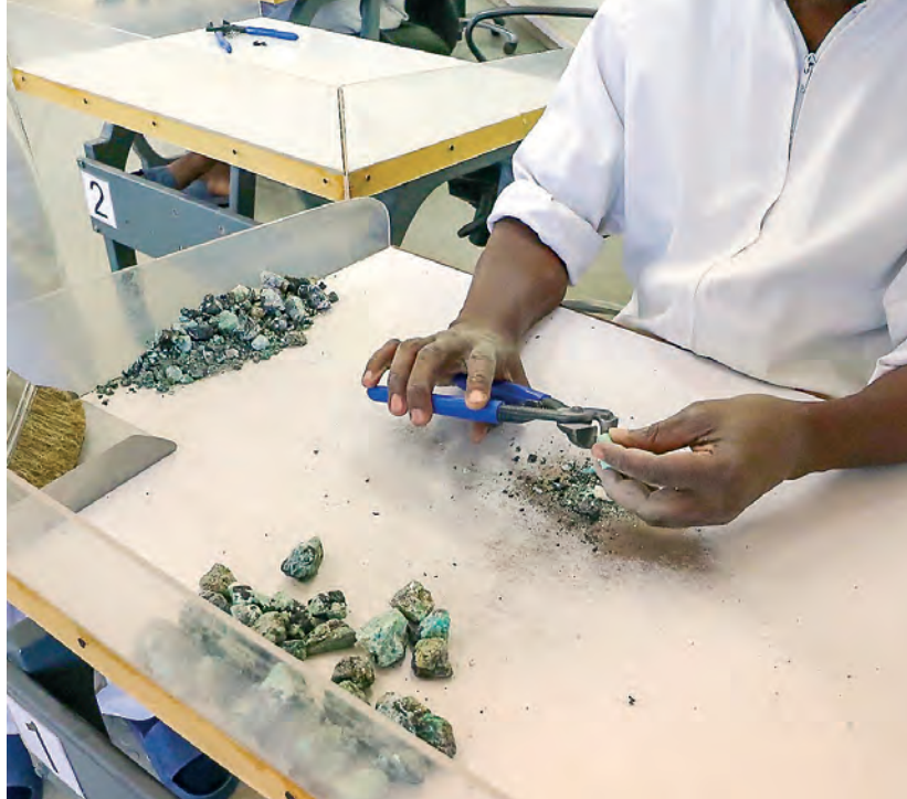
Chipping process in sort house.
